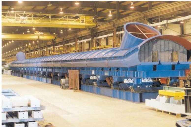
**Figure 7 Dynamically Balanced and Isolated Hot Solids Conveyor with Sealed Hoods**
