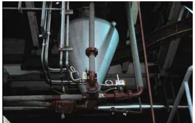
Figure 14 Typical DAC Dense Phase Transmitter
