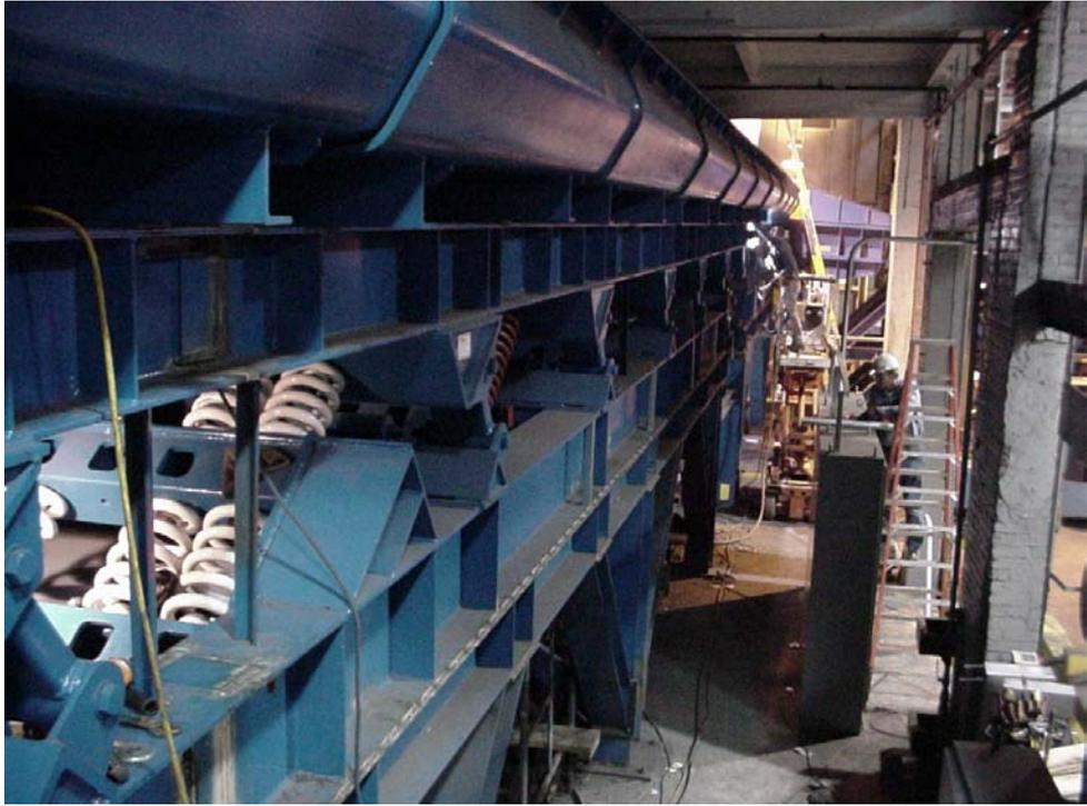
**Figure 8 Balanced and Isolated Conveyor with Provisions for Thermal Expansion**
