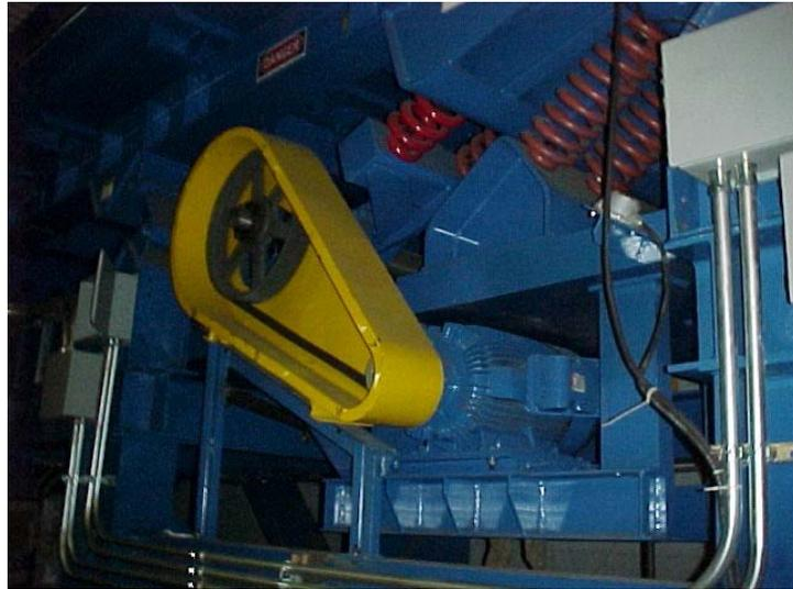
**Figure 10 Dynamically Balanced and Isolated Conveyor Drive**
