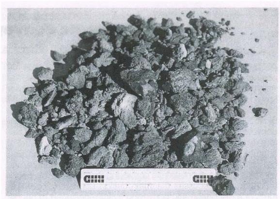
**Figure 3** Bottom ash from Florida Power's Crystal River Plant
