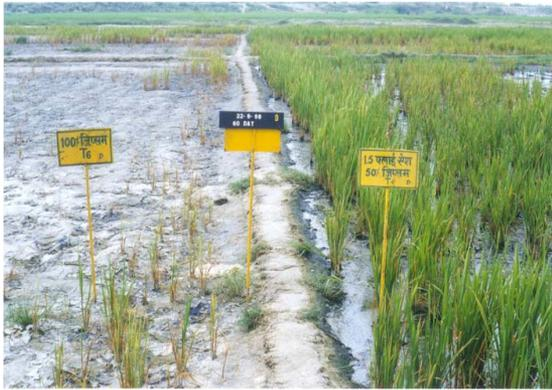
Reclamation of saline soils using fly ash (75% savings in Gypsum)
